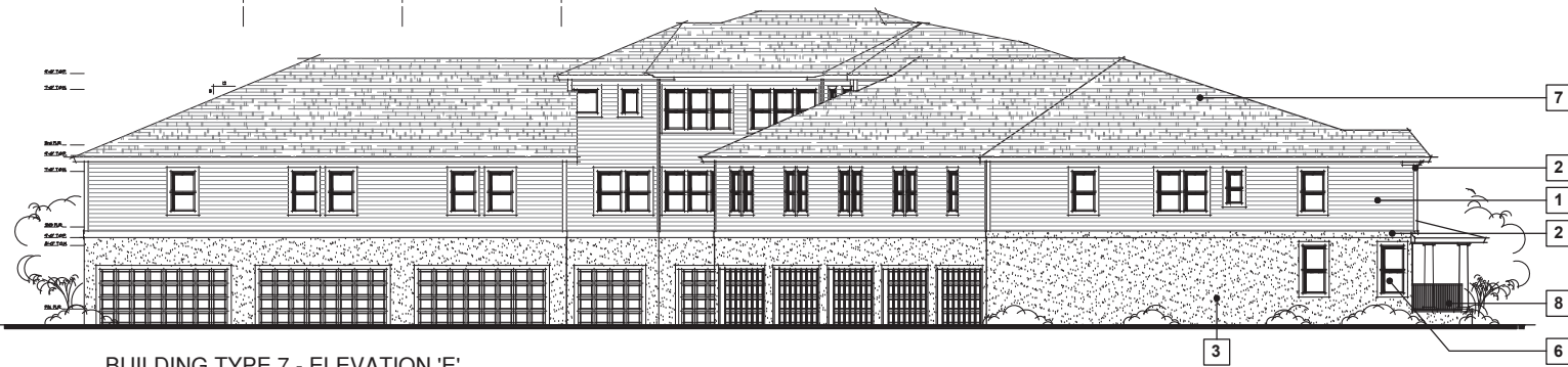
BUILDING TYPE 7 - ELEVATION 'E'
