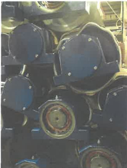
Charter design, one piece design with bolted plate. No place for rust to start.
