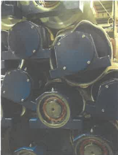
Charter design, one piece design with bolted plate. No place for rust to start.
